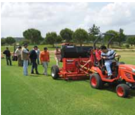
Descompactador-arejador Greens Terra Spike, de 1,60m + tractor KUBOTA BX 2350
